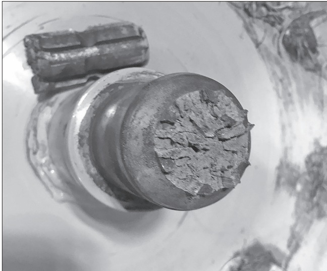
Broken Shaft From Severe Driveshaft Angle
