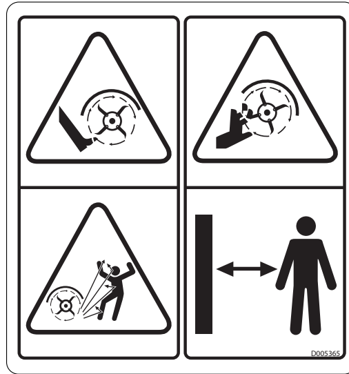
C. D005129 ⚠ WARNING - Rotating parts hazard. Do not reach into machine. Keep away from machine.
