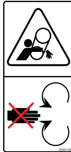
C. D005129 ⚠ WARNING - Rotating parts hazard. Do not reach into machine. Keep away from machine.
